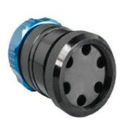
**Spider Clamp-** The P3-19 pin Spider Clamp offers cable strain relief combined with watertight sealing when using 6 individual cables in breakout applications. The design incorporates our "Spider Trap" mechanical grip mechanism which individually grips each cable jacket. The trap can be quickly and easily orientated to facilitate different cable diameters. A separate silicone grommet ensures a watertight assembly.
