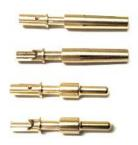
**Contacts**- Contacts are screw machined copper alloy with a gold plated finish. The multipoint contact design ensures low contact resistance and optimal current carrying capacity. Suitable for wire sizes 12-14AWG (1.5-2.5mm<sup>2</sup>).
